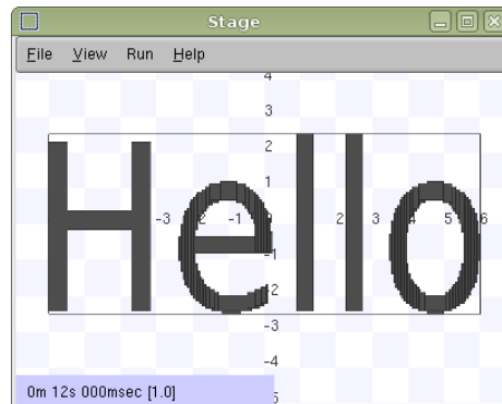
Figure 3.4: The left image is our "helloworld.png" bitmap, the right image is what Player/Stage interprets that bitmap as. The coloured areas are walls, the robot can move everywhere else.
